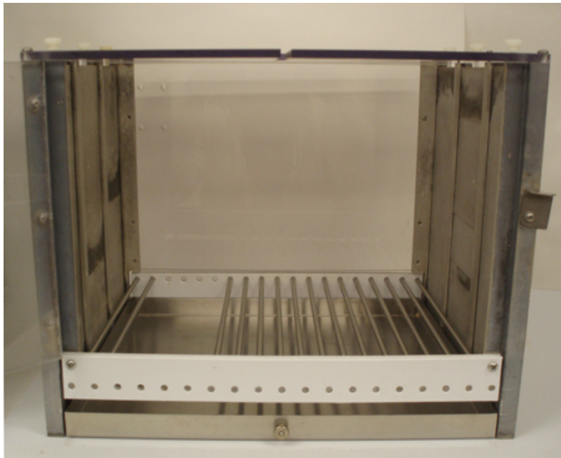
Figure 1. Testing in our laboratory was conducted in a bank of standard operant chambers (Med Associates Inc.) that were adapted for use in this task by removing four consecutive floor-bars to open up space for two scent cups.
