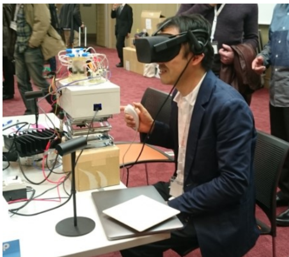
Figure 9: Application of the SAW atomizer coated with amorphous Teflon film. Research demonstration from the Intelligent User Interfaces (UI) Symposium 2018 in Tokyo, Japan.
