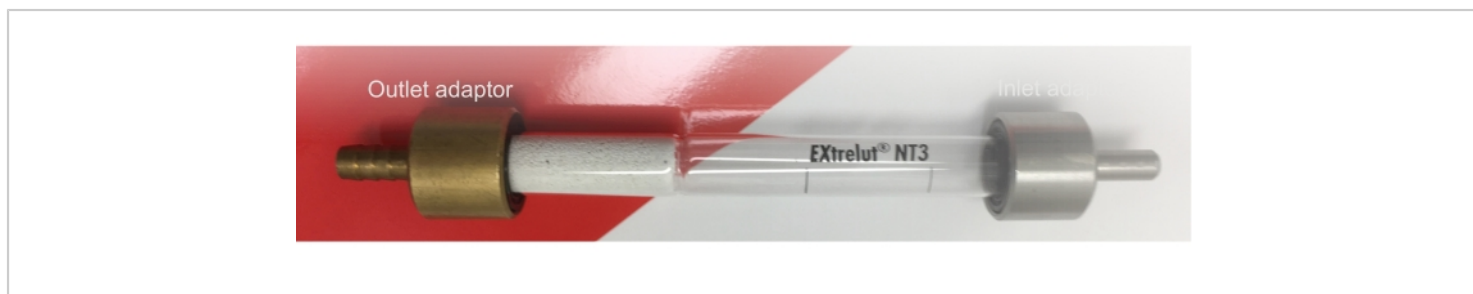
Figure 6: Sample column with attached adaptors. Before sampling, the sample column is preconditioned with 0.5 M sulfuric acid for nicotine analysis or isopropanol for flavor analysis. The inlet adaptor is connected to the CAG-generated aerosol flow and the outlet adaptor to the vacuum pump. Please click here to view a larger version of this figure.
