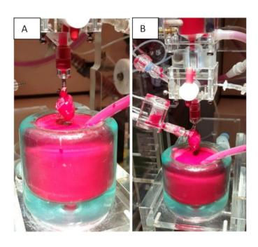
**Figure 3: Isolated heart apparatus.** (**A**) Langendorff mode. The heart is mounted to the WH apparatus via cannulation of the aorta. (**B**) Working heart mode. The system can be switched to the WH model to evaluate cardiac function by cannulating the left atrium. Please click here to view a larger version of this figure.
