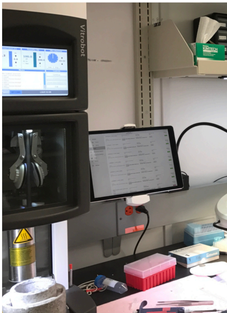
Figure 1. gP2S running on an iPad at a vitrification lab bench. The user interface has been designed for operation using touch screens, which facilitates in-lab use and accurate metadata entry. Please click here to view a larger version of this figure.
