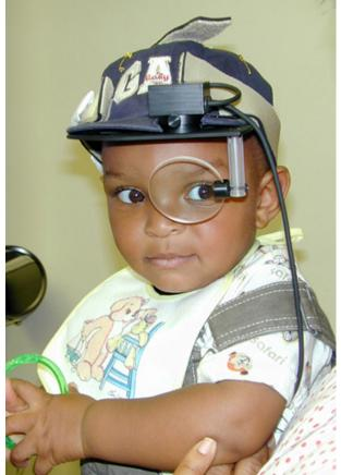
Figure 1. A head-mounted eye-tracking system.
