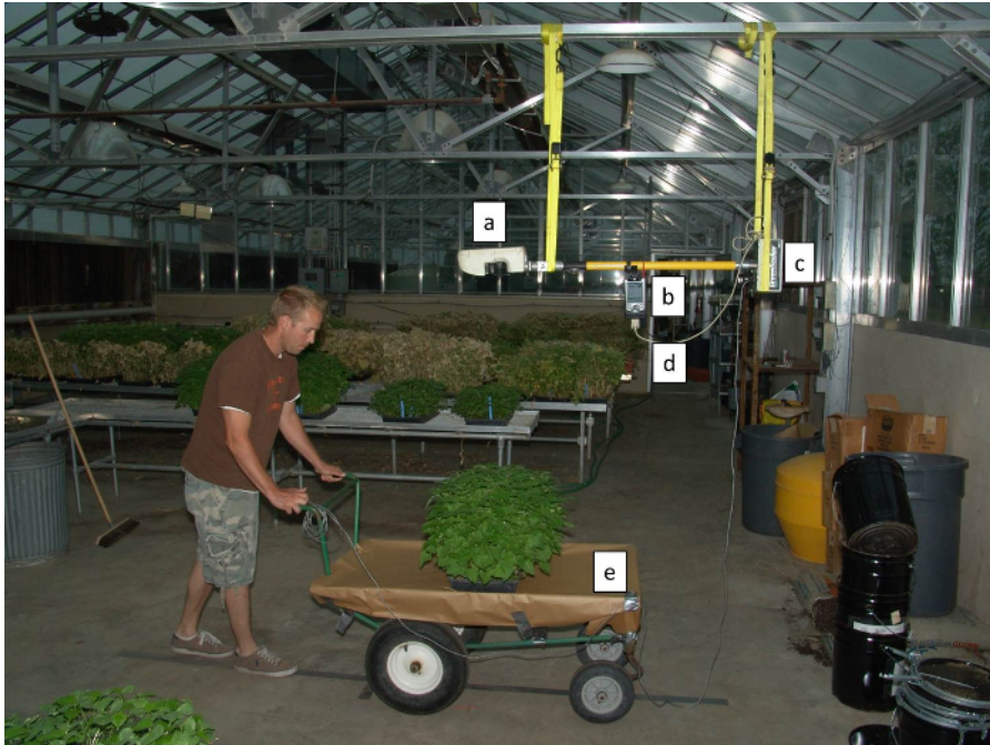
Figure 8. A multispectral optical sensor used to quantitatively measure the health of cotton plants infested with varying density levels of TSSM. The wheeled push cart with the test plants were slowly traversed under the sensor head to obtain spectral reflectance values. a is the sensor head; b is pocket PC; c is battery compartment and input/output ports; d is RS-232 serial data cable and e is the craft paper to provide uniform background. Please click here to view a larger version of this figure.
