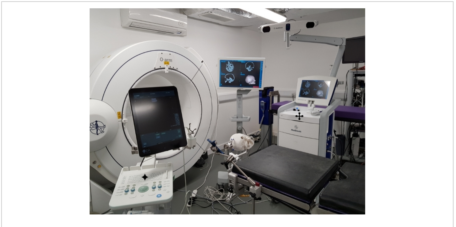
Figure 7: Testing the phantom during surgical simulation. Testing the phantom model through surgical simulation in a virtual operating room. ✚: neuronavigation system displaying the registered scan of the CT phantom model, ✚: ultrasound system used to image the phantom with a burr hole ultrasound transducer (seen positioned next to the ultrasound monitor). Note the model pictured here is based on data acquired from different patient with a right sided tumor. Please click here to view a larger version of this figure.
