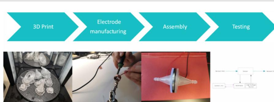
**Figure 3: Schematic for the method.** The protocol is divided into four major steps. First, all parts for the sensor housing are printed. Then, the electrodes are manufactured. In the third step, the 3D printed sensor housing with the electrodes and the vacuum gasket are assembled. In the last step, the sensor performance is evaluated. [Please click here to view a larger version of this figure.](#)
