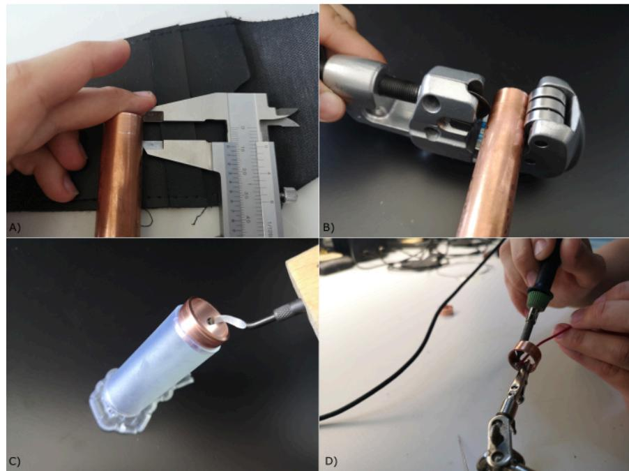
**Figure 5: Electrode manufacturing.** (A) Measuring, (B) cutting, (C) deburring, and (D) soldering of the electrodes. [Please click here to view a larger version of this figure.](#)
