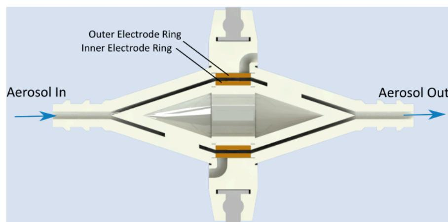
**Figure 1: Sensor schematics.** Aerosol flows into the aerosol inlet, is propagated through the left flow channel, and then reaches the gap between the high-voltage electrode (inner electrode) and the measuring electrode (outer electrode). There,
