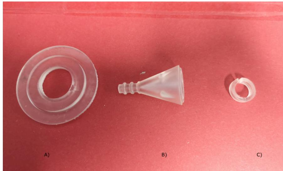
**Figure 6: Sensor parts.** (A) The outer electrode holder, (B) flow channel, and (C) the inner electrode holder. Please click [here](#) to view a larger version of this figure.
