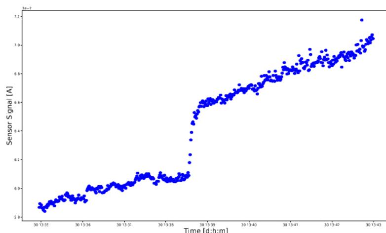
**Figure 12: Negative result.** A short circuit has occurred during the measurement. The sensor signal in amperes is plotted on the vertical axis and the measurement time is plotted on the horizontal axis. The sensor signal continues to increase without restriction. [Please click here to view a larger version of this figure.](#)
