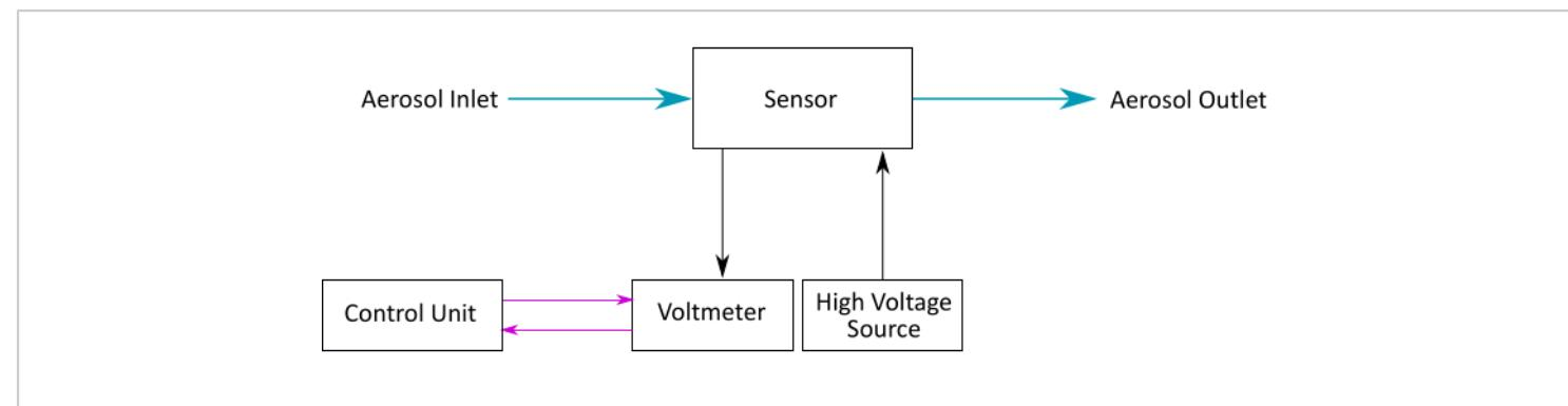
**Figure 8: Sensor setup.** A diagram of the sensor setup. Aerosol flows through the sensor. The sensor is connected to the voltmeter and a high-voltage supply. The voltmeter is controlled by a control unit that logs the sensor data. [Please click here to view a larger version of this figure.](#)
