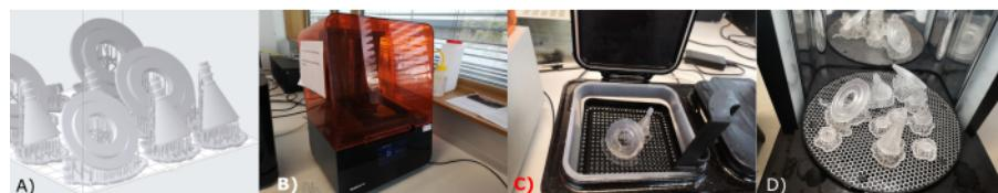
**Figure 4: Schematic of 3D print.** (A) The slicer 3D model is depicted; (B) the printer during the printing process. Postprocessing steps: (C) flushing and (D) UV-hardening. [Please click here to view a larger version of this figure.](#)
