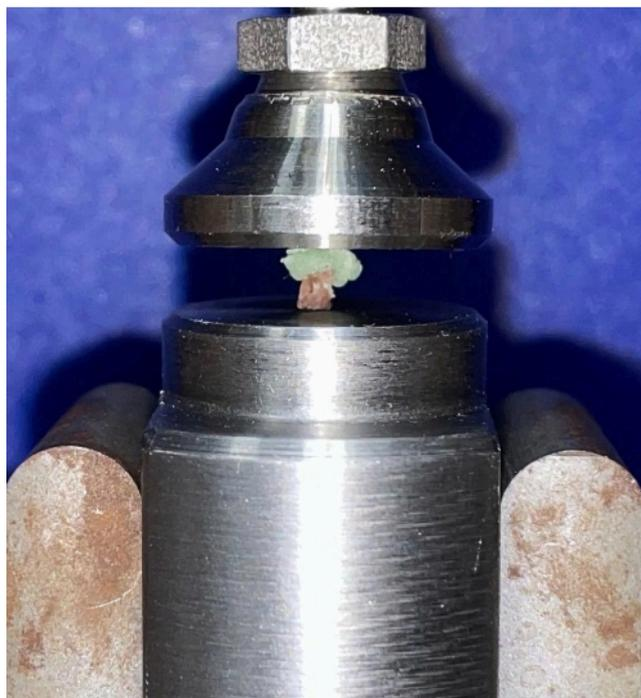
**Figure 5: Hardening period of PMMA bone cement.** An example L5 vertebra with PMMA bone cement (green) placed on the cranial endplate and the top platen lowered onto the PMMA bone cement + bone complex. Once PMMA bone cement has fully hardened, the compression test will begin. The top platen will be further lowered until failure of the material is observed. [Please click here to view a larger version of this figure.](#)
