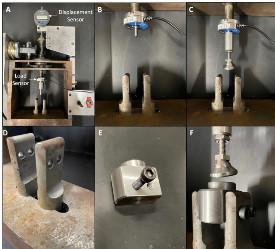
**Figure 1: The conversion of a three-point bending machine to a compression testing machine. (A)** The machine fully equipped to operate as a three-point bending machine with the displacement sensor and load sensor indicated (white arrows). **(B)** The machine after the crosshead beam has been removed. **(C)** The machine after a self-aligning top platen has been placed where the crosshead beam was previously placed. **(D)** The lower support beams with holes drilled into them. **(E)**
