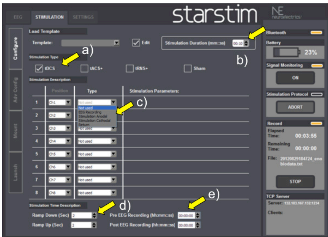
Figure 3. Stimulation Screenshot: a) Electrical stimulation mode (tDCS, tACS, tRNS, sham); b) Total duration of electrical stimulation; c) Electrode positioning according to channels; d) tDCS and EEG channel configuration; e) tDCS ramping duration; f) EEG recording durations.
