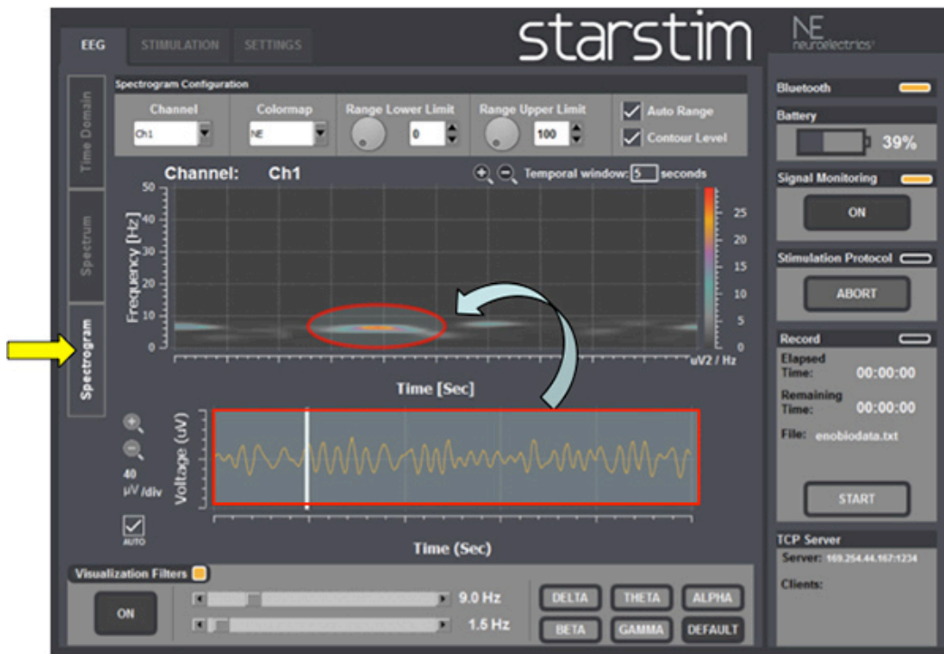
Figure 8. EEG spectrogram: EEG signals (red rectangle on the bottom) can also be transformed into images (red circle) using a technique called time-frequency based.
