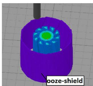
**Figure 4: Virtual print of a component with surrounding ooze-shield.** [Please click here to view a larger version of this figure.](#)
