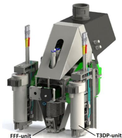
**Figure 16:** CAD model of new print head with two FFF-printing heads and two T3DP-printing heads. [Please click here to view a larger version of this figure.](#)
