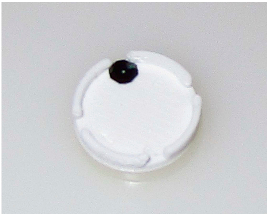
Figure 2: Photograph of 3D printed adapter, used to hold the TEM membrane off-axis during the spin coating. Multiple membranes can be coated at the same time. Please click here to view a larger version of this figure.
