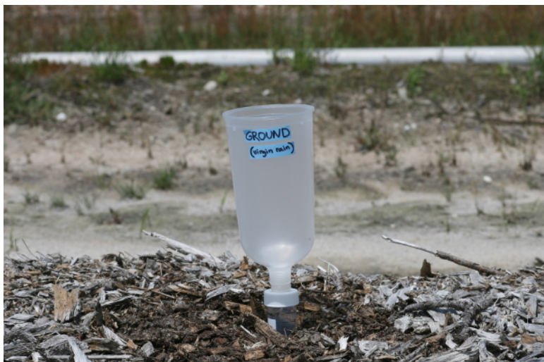
Supplemental Figure 6: Blueberry rainwater deployment (ground). Completed virgin rainwater collection device, placed adjacent to blueberry bushes. Please click here to view a larger version of this figure.
