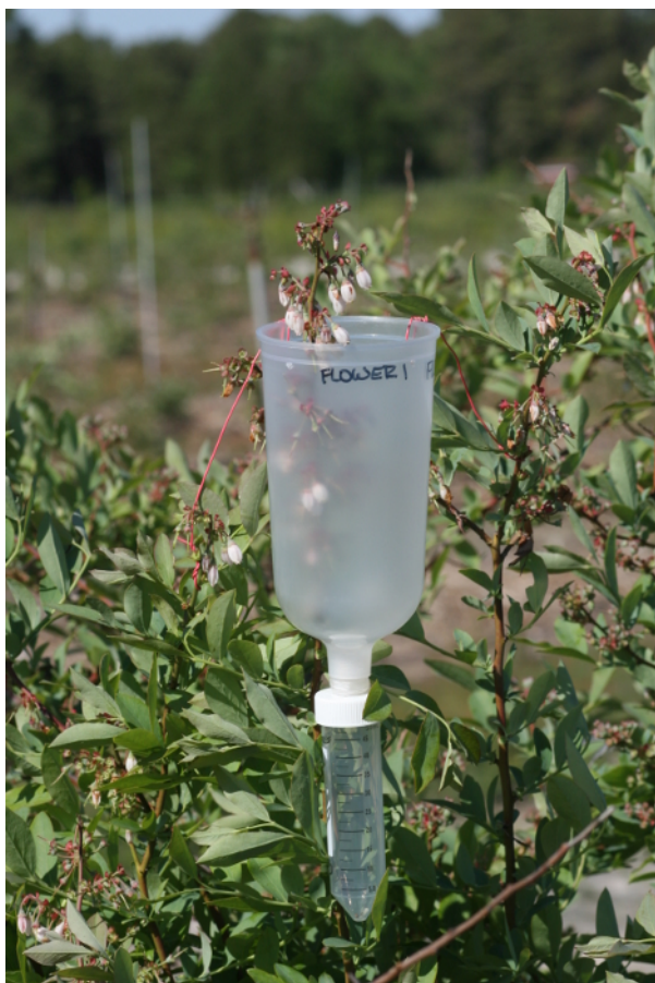
Supplemental Figure 3: Blueberry rainwater deployment (flower). Completed blueberry floral rainwater collection device, placed directly under a cluster of inflorescences. Note the plastic-coated wire used to vertically orient the device. Please click here to view a larger version of this figure.
