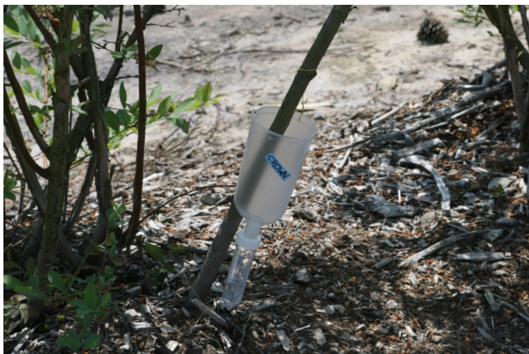
Supplemental Figure 5: Blueberry rainwater deployment (crown). Completed blueberry floral rainwater collection device, placed at the base of the bush (crown). Note plastic coated wires can be removed if not necessary. Please click here to view a larger version of this figure.
