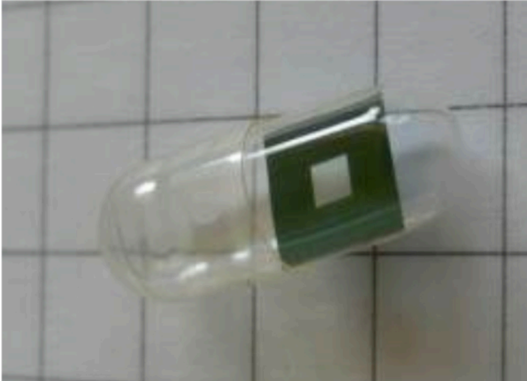
Figure 1: Typical sample support for X-ray fluorescence nano-analysis. A \text{Si}_3\text{N}_4 membrane support in its protective capsule. This type of substrate can be used both for room temperature analysis (plunge-freeze cellular preparation followed by low temperature and low vacuum freeze-drying process) or for cryogenic X-ray fluorescence analysis. Please click here to view a larger version of this figure.
