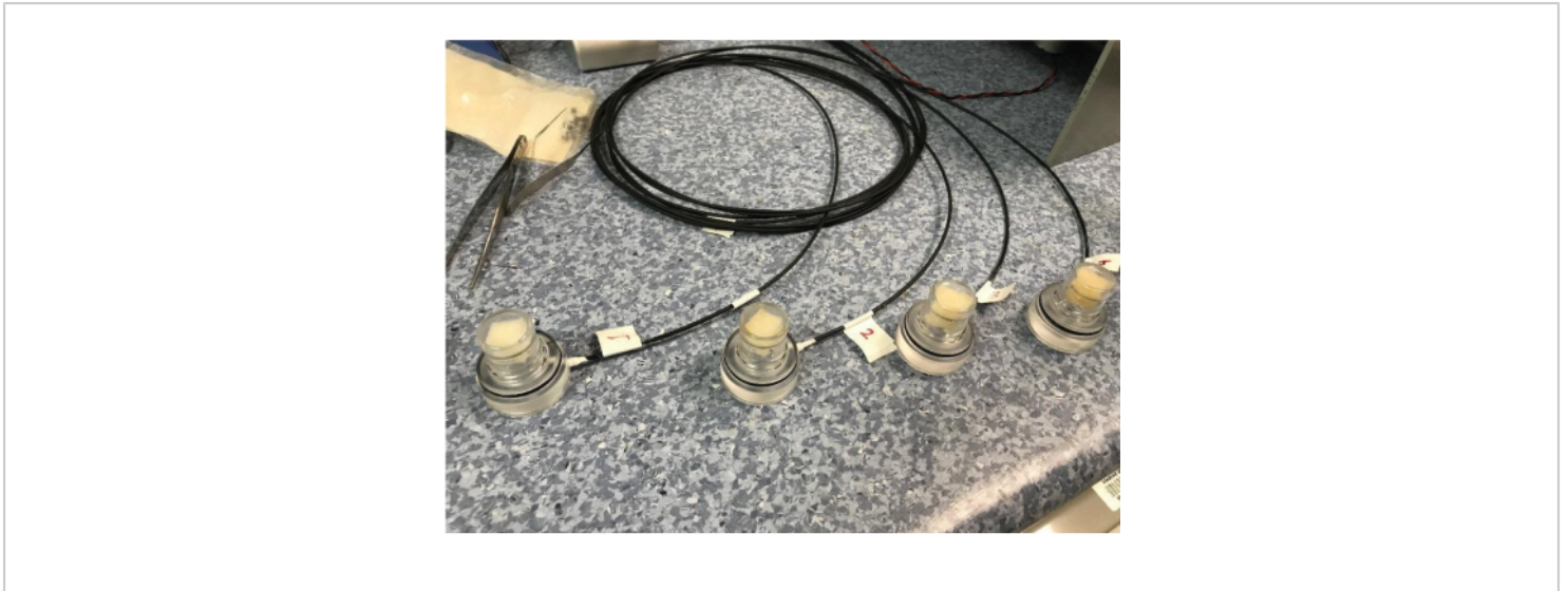
Figure 6: Chambers placed upside down, ready for calibration. Please click here to view a larger version of this figure.
