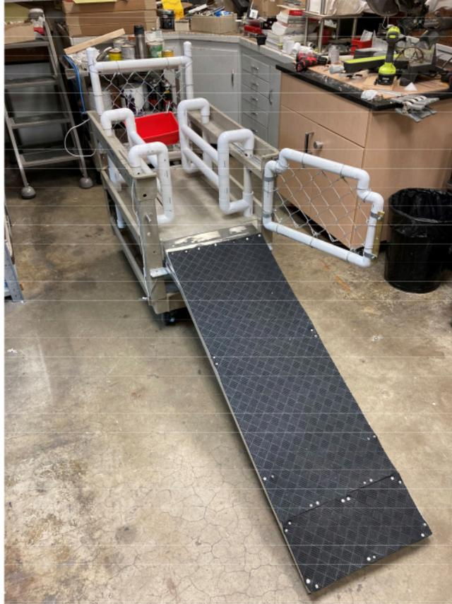
**Figure 4: Aluminum ramp.** An aluminum ramp is attached to the front or back of the cart, and removable rubber padding is added for grip using bolts and grommets. [Please click here to view a larger version of this figure.](#)
