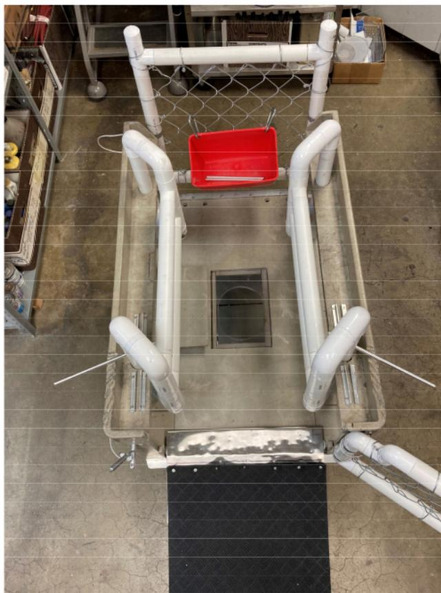
**Figure 3: Top view of the echocardiography cart.** An aperture is created on the top floor of the cart for passing a hand holding an ultrasound probe. A plastic over-piece is fitted for safe cart mounting and dismounting. [Please click here to view a larger version of this figure.](#)
