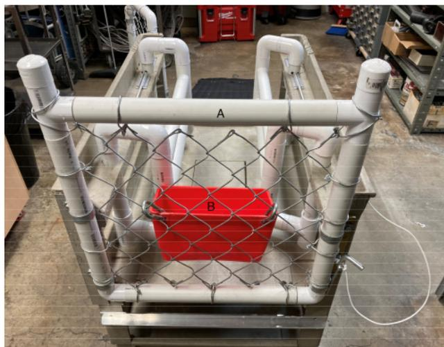
**Figure 2: Head view of the echocardiography cart.** The front and back of the pre-made cart are replaced with hinged gates made of PVC pipe and chain link (**A**), which also accommodates a hanging food trough (**B**). [Please click here to view a larger version of this figure.](#)
