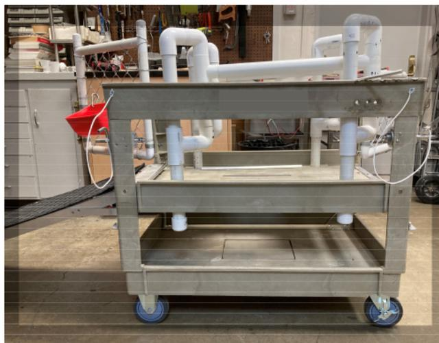
**Figure 1: Side view of the echocardiography cart.** The echocardiography cart is built using a pre-made heavy-duty utility cart. [Please click here to view a larger version of this figure.](#)
