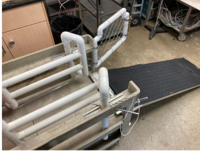
**Figure 5: Side gate.** Hinges are created for the side gates, with pins to allow for more accurate sizing and restraint. [Please click here to view a larger version of this figure.](#)
