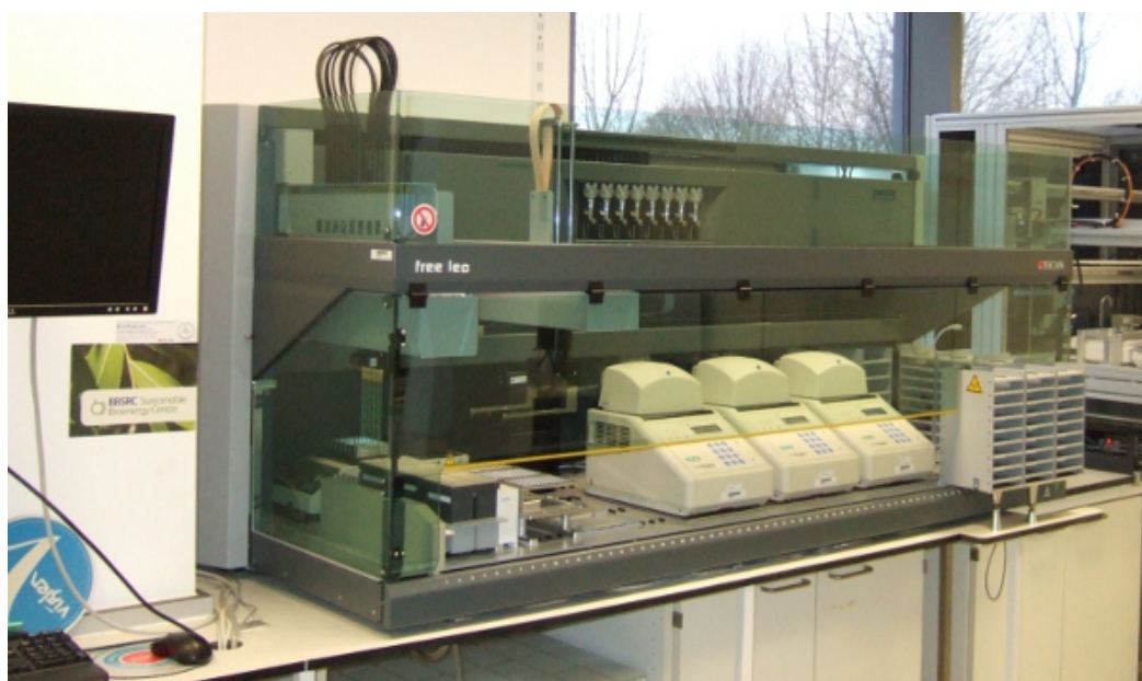
Figure 2. Liquid handling station for the High Throughput saccharification analysis
