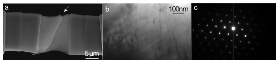
Figure 6: A representative Single crystal copper (SSC) specimen. (a) shows the gauge section (location A from Figure 1) taken after failure of the gauge section. (b) is a bright field image of the gauge section showing plane dislocations. (c) shows the diffraction pattern at the gauge section. Modified 13 , with the permission of AIP Publishing. Please click here to view a larger version of this figure.
