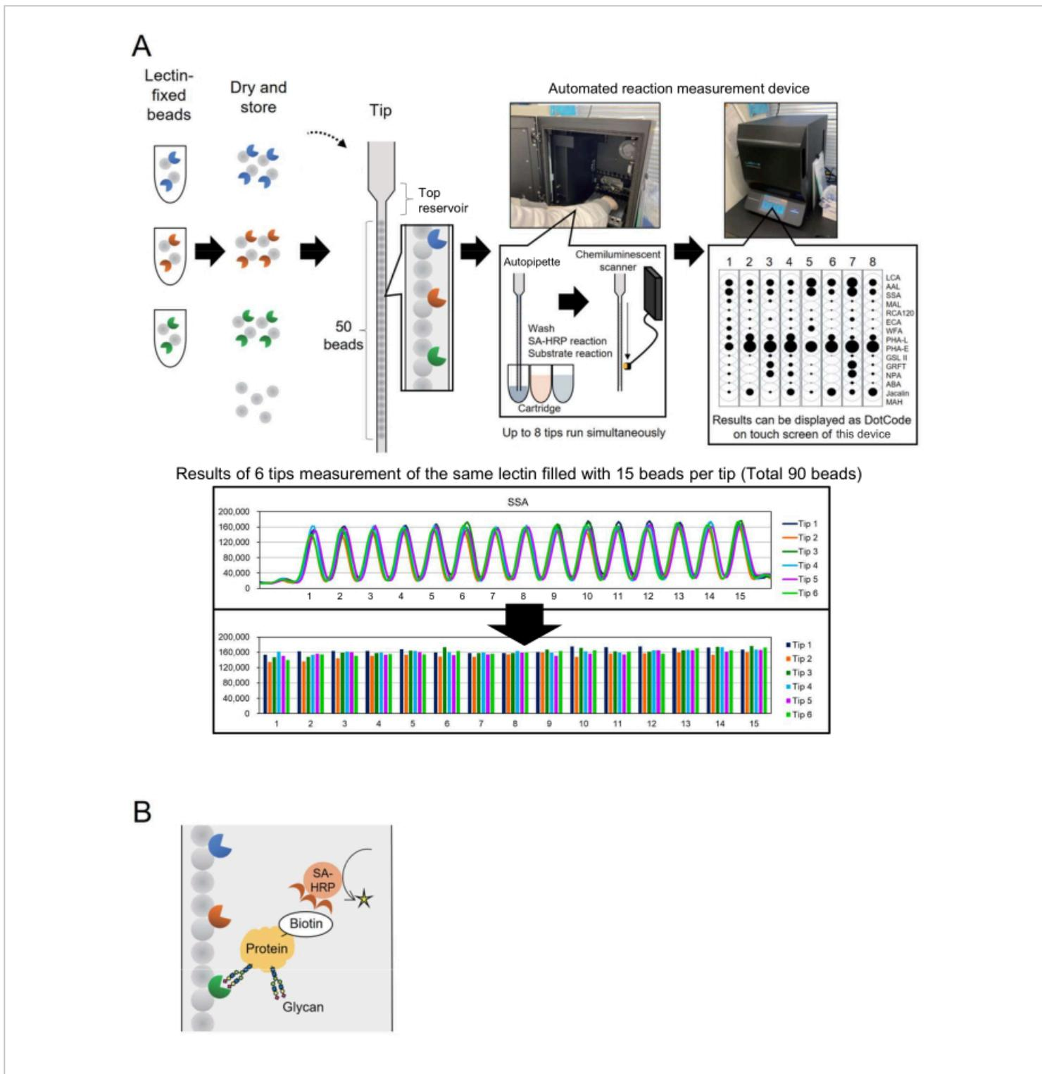
**Figure 1: Schemes of the "bead array in a single tip" instrument and analysis method. (A)** Scheme of automatic glycan profiling system. Lectin-fixed beads can be dried and stored in tips. When tips and cartridges containing reagents like HRP-labeled anti-streptavidin antibody (SA-HRP) are set in the measuring instrument (automated reaction measurement device) and activated, the tip functions as an autopipette. The chemiluminescence detection scanner at the instrument's
